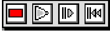
Figure 9. The Control Panel buttons can be used to control the running of the simulation. From left to right, the buttons are "Stop," "Go," "Step," and "Reset." These commands are also available from the Control menu.
