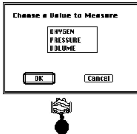
Note that, once attached, the gauge may be dragged away from the connection point without breaking the connection; a solid line between the gauge and its
